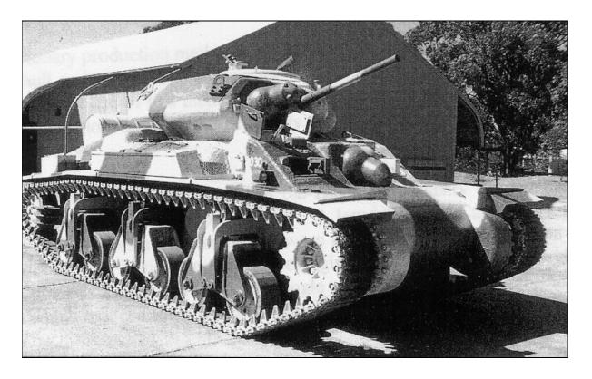
The pilot model of the Sentinel was completed in March 1942 and by August 1942, the first production tank was completed in the NSW Railway Workshops. The first Sentinel Mk I weighed 26 tons, mounted a 2-pr (40 mm) gun and two Vickers machine guns. The frontal armour was 65 mm and the vehicle achieved a top speed of 48 km/h.
