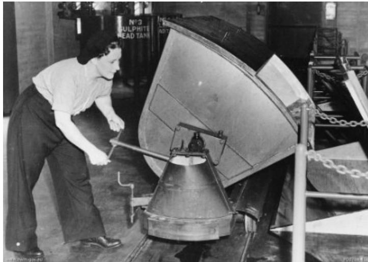
1944. A woman operates a machine which tips crude TNT into a chute which leads to the wash vats for converting to liquid TNT.
